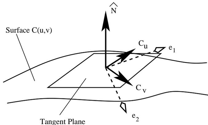
Figure 1: Relationship of tangent plane and normal vectors in determining curvature.  $\mathbf{C}_u$  and  $\mathbf{C}_v$  are derivatives of surface with respect to parameters  $u, v$ . Normal  $\hat{\mathbf{N}} = \frac{\mathbf{C}_u \times \mathbf{C}_v}{|\mathbf{C}_u \times \mathbf{C}_v|}$ .  $\mathbf{e}_1, \mathbf{e}_2$  are eigenvectors of Weingarten mapping matrix  $\mathbf{H}$ .
